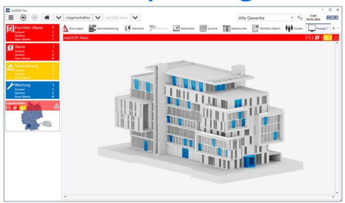
Building management system for visualisation, operation, control and monitoring of connected GEZE product systems
