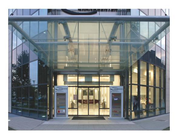
Automatic linear sliding door system with burglar resistance in accordance with resistance class RC2
